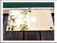
**CK-AF COATED SIDE SWIPED CLEAN** Using a simple soft galley sink sponge, the remaining plant growth is easily removed, facilitated by the lubricious, hard ceramic surface. The original coated surface is revealed. There were never any algae or barnacles formed on this coated side. Boat bottom is ready to go another 3-4 weeks, or longer, before the next cleaning. A dream for boat bottom cleaners!
