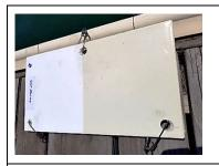
**BEFORE IMMERSION** The test sample is coated with CK-AF on the right and has no coating on the left, just bare fiberglass. It is then lowered to 24" below the waterline in San Diego Bay.
