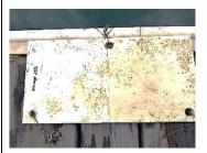
**AFTER 3 WEEKS IMMERSION** Some marine plant life is beginning to grow on the coated right-hand panel; there is no algae. The left-hand uncoated section has algae beginning to form plus some minor hard marine growth (barnacles).
